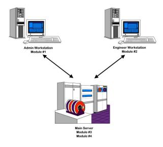
Engineer's workstation respectively. The Data Modules #3 & #4 are installed together on the company's Main Server or a Department Dedicated Server. Regardless, it is very important that the data on the server is backed up regularly to protect data integrity.
